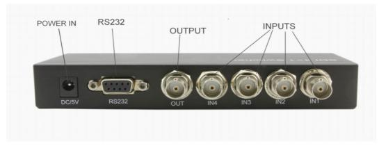
Power in, DC 5V/2A adapter available; RS232 interface, connect to computer system; Four SDI inputs connect to SDI source, such as SDI Camera; One SDI output connects to SDI monitor or other SDI Device.
