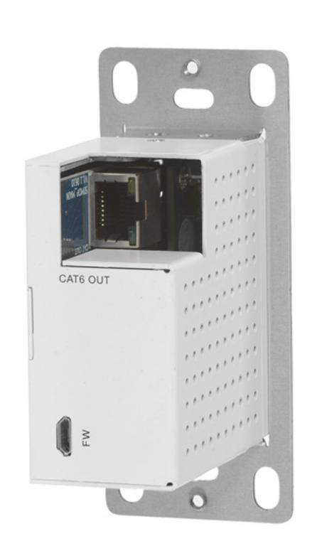
The KanexPro WP-EXTHDTC50 HDMI and USB-C 50M Extender Wall Plate kit is a 2x1 switcher and transmitter with HDMI and USB-C inputs. It features a US one-gang enclosure for Decora-style wall plate opening with white wall plates and faceplates. Supports video resolutions up to 4K2K@50/60Hz 4:4:4. The RJ56 output can extend video transmission at distances up to 164ft or 50m. The wall-plate transmitter is remotely powered by the receiver via POC technology.
