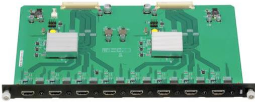
**FLEX-HDMI8IN: 8 ports HDMI Input Card**
