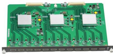
**FLEX-HDMIOUT: 12 ports HDMI Output Card**
