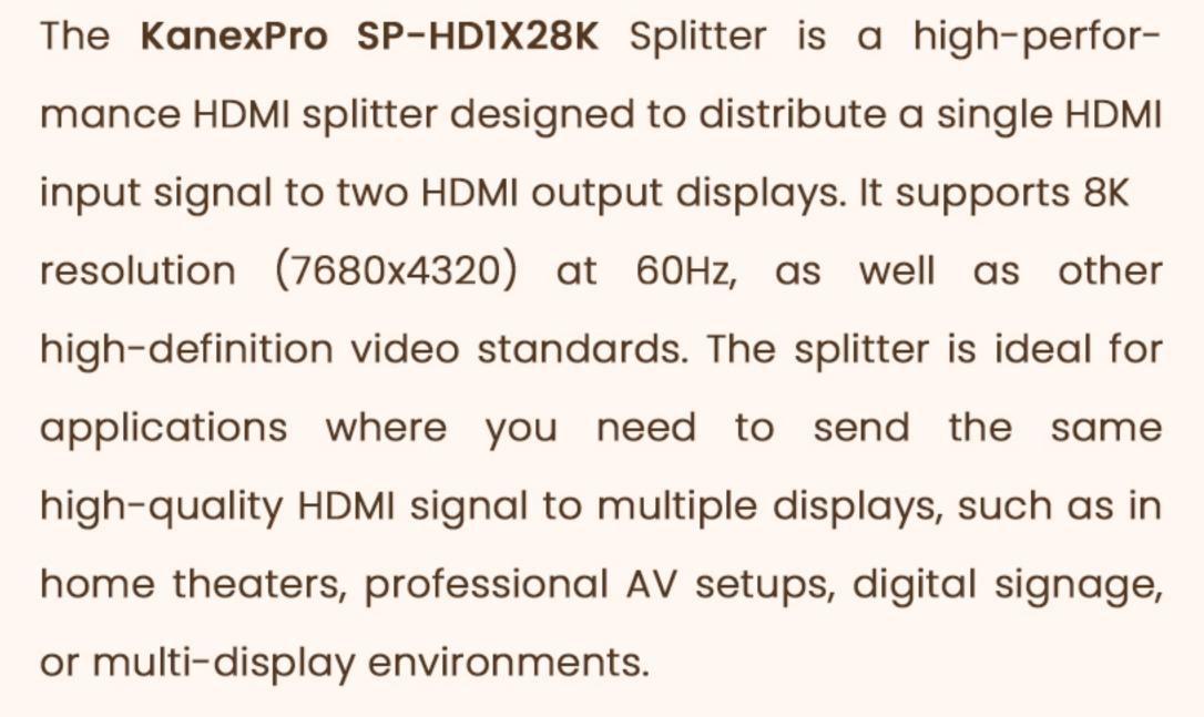
The KanexPro SP-HD1X28K 1x2 splitter is an advanced solution for splitting single HDMI signal to 2 HDMI outputs synchronously, with video resolution up to 8K@60 4:2:0 12bit. It supports data rates up to 48Gbps to comply with HDMI 2.1 and HDCP 2.3 requirements. It includes several features for ease of integration, including EDID management, cable equalization. This multi-functional product can work well with X-box or PS5 to achieve 4K@120Hz on your TVs or relative monitors.
