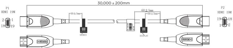
50M (164FT) 50,000 ± 200mm P2 P1  $60 \pm 5$ mm HDMI 19M HDMI 19M -50±5mm- $-50 \pm 5$ mm-19-18 2-**1** 18**1**9 DISPL 38  $_{1}$ PRI : 1400 A010M SOURCE DISPLAY (wer
