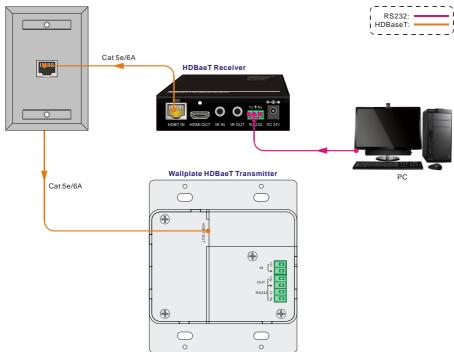
The RS232 control mode can be chosen via RS232 commands, please refer to the **5.3.1 RS232 mode switching** for more details.
