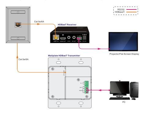
② Control the Wallplate HDBaseT Transmitter by the remote PC which relates to Receiver
