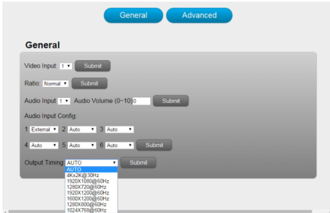
HDMI output resolution selection: AUTO (auto adjustment of the output resolution based on the EDID of the display device), 4Kx2K@30Hz, 1920x1080@60Hz, 1280x720@60Hz, 1920x1200@60Hz, 1600x1200@60Hz, 1280x800@60Hz, 1024x768@60Hz. Select the related parameters, and click **Submit** to make the changes take effect.
