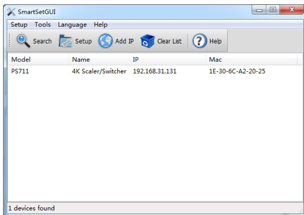
Select the device, and click **Setup**. The IP information is obtained from the **Device Info** page:
