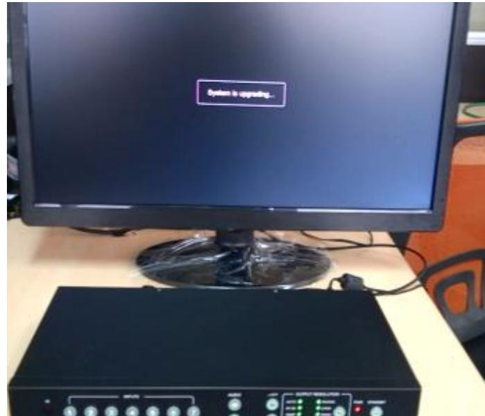
Attention: The unit can't be power-off until the upgrading progress is finished. Or, the unit firmware will be corrupted.
