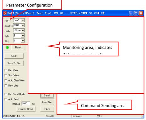
Please set the parameters of COM number, bound rate, data bit, stop bit and the parity bit correctly, and then you can send command in Command Sending Area.
