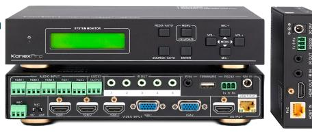
The KanexPro HDSC51HDBT is a mini hi-def. presentation scaler designed for installation beneath conference tables and in lecterns to provide localized audio and video switching support for sources such as presenter devices, as well as signal extension up to 230 feet over shielded CAT6 cable to reach a wall or ceilingmounted display using HDBaseT.
