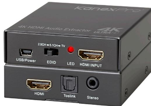
The KanexPro HAECOAX2 is a 4K compliant audio de-embedder that extracts the audio from HDMI signal and provides outputs for analog stereo using 3.5mm head phone jack and digital TOSLINK audio.
