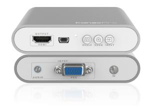
**The KanexPro CON-VGA-HD4K** is a universal scaler converter designed to up-scale one VGA (15-pin HD) input to HDMI 4Kx2K@60Hz output. The CON-VGA-HD4K is capable of converting analog to digital formats with multiple adjustments and range to achieve the most ideal video image. Its portable and simple plug and play functionality making it the most ideal scale converters for analog to 4K digital signal conversion.
