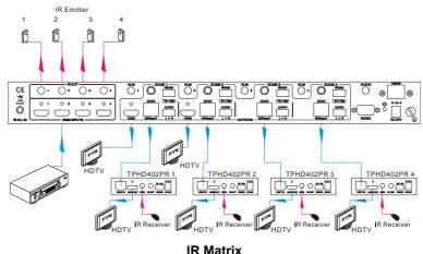
The IR signal is sent by corresponding IR remote, then it is transferred to HDBaseT receiver, then to corresponding zone of the matrix through the twisted pair, finally it is transferred to IR OUT port and received by controlled device.
