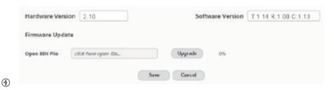
Upload new firmware versions and see current ones install. This can update the firmware of the control panel and the receiver box, not the two-gang transmitter. To update the firmware of the two-gang switcher, use the USB port on the plate.
